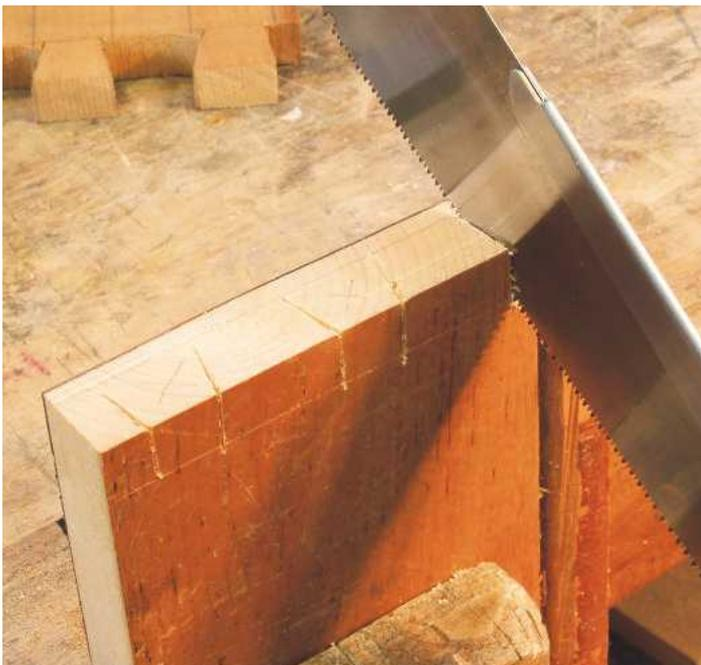
▲ Pic.8 Cutting the lapped pins
